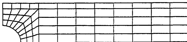
Fig. 6. Mesh for the circular inclusion problem.
